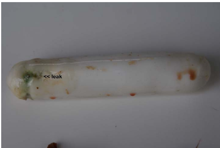
Figure 2. Leak in a transmitter
