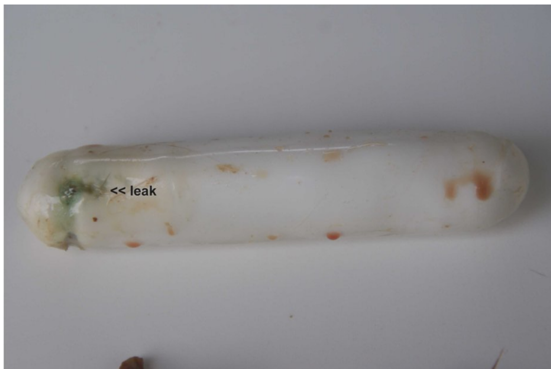
Figure 2. Leak in a transmitter
