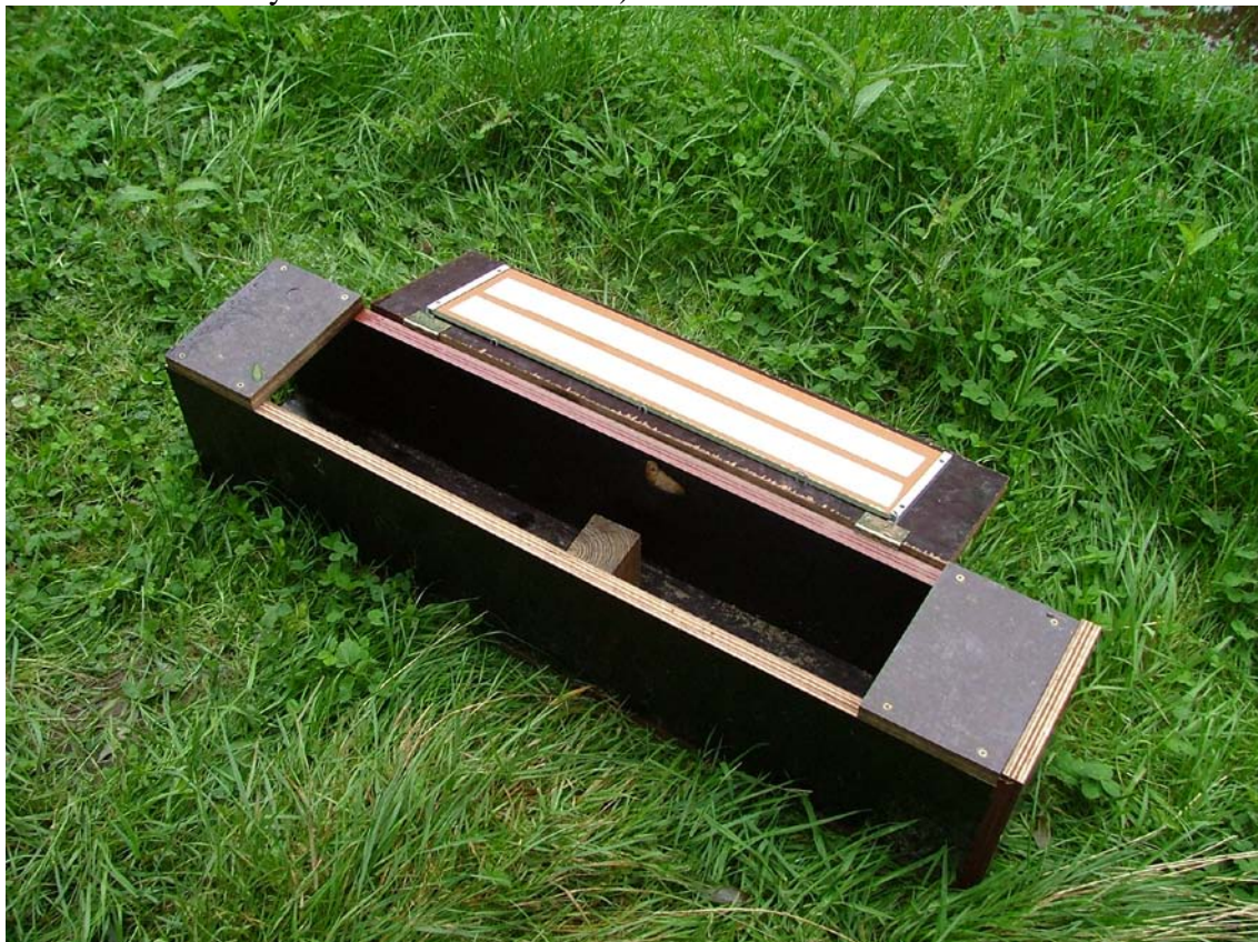
Figure 1. Wooden box with double sided adhesive tape on a removable board
